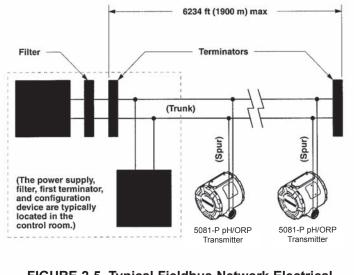
FIGURE 2-5. Typical Fieldbus Network Electrical Wiring Configuration
