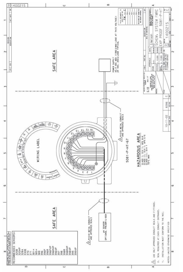
FIGURE 4-3. FM Explosion-Proof Installation for Model 5081-P-HT
