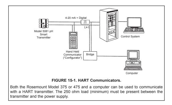
If your communicator does not recognize the Model 5081-P pH/ORP transmitter, the device description library may need updating. Call the manufacturer of your HART communication device for updates.
