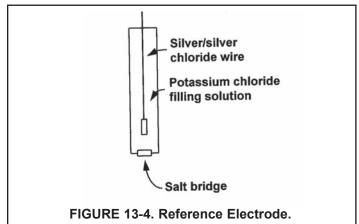
The fixed concentration of chloride inside the electrode keeps the potential constant. A porous plug salt bridge at the bottom of the electrode permits electrical contact between the reference electrode and the test solution.
