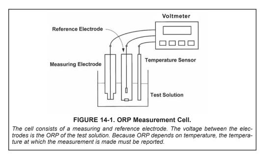
Figure 14-1 shows separate measuring and reference electrodes. In most process sensors the electrodes and the temperature element are combined into a single body. Such sensors are often called combination electrodes.
