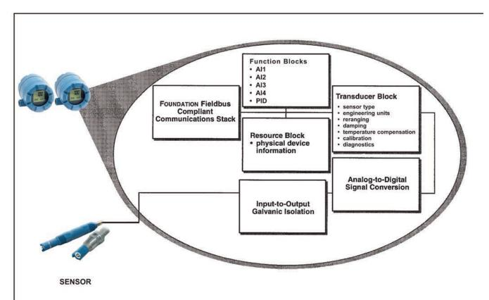
FIGURE 5-1. Functional Block Diagram for the Model 5081-P pH/ORP Transmitter with FOUNDATION Fieldbus.
