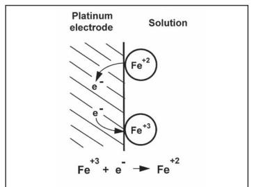
FIGURE 14-5. Electrode Potential.
