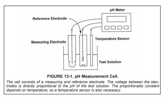
Figure 13-1 shows separate measuring and reference electrodes. In most process sensors, the electrodes and the temperature element are combined into a single body. Such sensors are often called combination electrodes.
