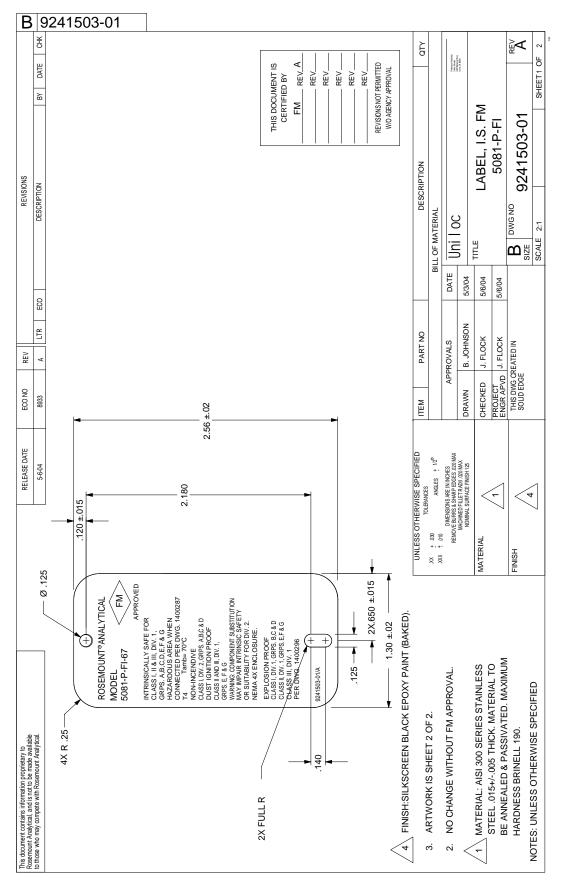
FIGURE 4-15. FM Intrinsically Safe Label for Model 5081-P-FI
