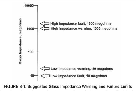
Typical glass impedance is about 100 megohms at 25°C. A broken electrode has an impedance of 10 megohms or less. A glass impedance greater than 1000 megohms suggests the electrode is nearing the end of its service life. High impedance may also mean the electrode is not immersed in the process liquid.
