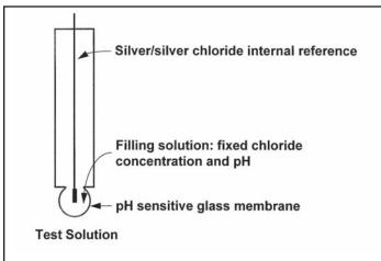
FIGURE 13-2. Measuring Electrode.
