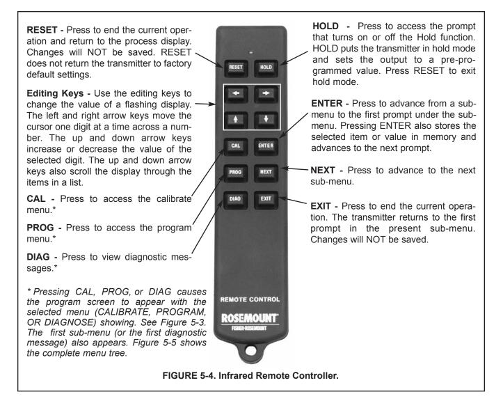
Hold the IRC within 6 feet of the transmitter, and not more than 15 degrees from horizontal to the display window.
