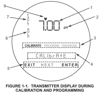
The program display screen allows access to calibration and programming menus.
