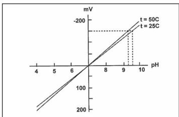
FIGURE 13-6. Glass Electrode Slope.
