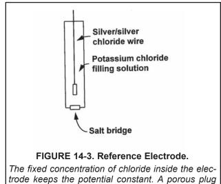
trode keeps the potential constant. A porous plug salt bridge at the bottom of the electrode permits electrical contact between the reference electrode and the test solution.
