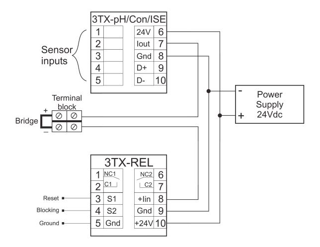
If you wish to "insert" an external device into the current loop, it can be done by removing the bridge jumper and connecting the two terminals to the external device ("+" to device input and "-" to device output, which may also be device ground). If no external device is to be connected, the bridge jumper must be in place to ensure normal operation of the 3TX-REL relay module.
